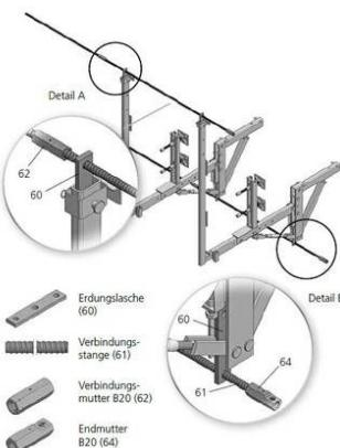
For grounding the canopy framework over electrified railroad lines.
