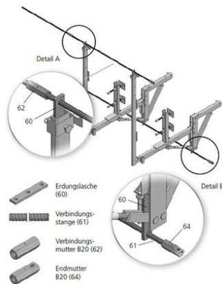
For grounding the canopy framework over electrified railroad lines.
