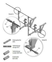
For grounding the canopy framework over electrified railroad lines. Approval of the DB available.
