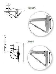
For height adjustment and inclination adjustment of the formwork beam.
