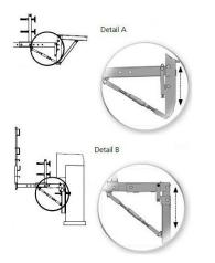
For height adjustment and inclination adjustment of the formwork beam.
