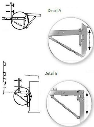
For height adjustment and inclination adjustment of the formwork beam.
