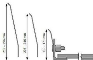
Cap formwork, on the roadway side with height-adjustable sheet steel on a carrier profile for curb formation in accordance with RiZ-ING Chapters 1-5, 6, 7, 9 and 10. Additional component: S-carrier extension 200 to avoid penetration of the seal in the curb area when dowelling.
