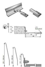
Cap formwork, on the roadway side with height-adjustable sheet steel on a carrier profile for curb formation in accordance with RiZ-ING Chapters 1-5, 6, 7, 9 and 10. Additional component: S-carrier extension 200 to avoid penetration of the seal in the curb area when dowelling.
