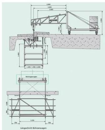
This combination is used especially in the area of the central cornice. The stage platform offers ideal conditions for assembly work and visual inspections under the bridge. The flow of traffic on the side of the bridge that is being used is not affected.
