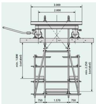
Mobile work platform for the efficient installation of BETOMAX® cornice consoles and pipelines or inspection views or renovation work under the central cap areas of bridge superstructures that are close together.
