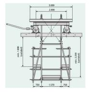
Mobile work platform for the efficient installation of BETOMAX® cornice consoles and pipelines or inspection views or renovation work under the central cap areas of bridge superstructures that are close together.
