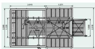
Mobile work platform for sighting and renovation work, assembly/disassembly of cornice consoles or laying of pipelines in bridge edge areas.
