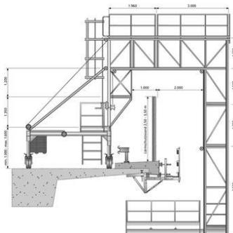
Mobile work platform for special applications, e.g. B. Refurbishment and new construction, especially for buildings with existing noise protection walls max. 3.50 m:
