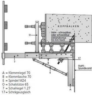
With the BETOMAX® sheet piling bracket 2000/70-s it is possible to produce head beams on sheet piling profiles safely and efficiently. All the advantages of the BETOMAX® cornice bracket 2000 in terms of adjustment options and safety devices (e.g. walkway with railing posts) can be used.
