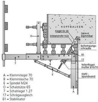
With the BETOMAX® sheet pile bracket 2000/70-k it is possible to produce head beams on sheet pile profiles safely and efficiently. All the advantages of the BETOMAX® cornice bracket 2000 in terms of adjustment options and safety devices (e.g. walkway with railing posts) can be used.
