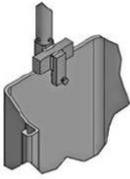
Railing post holder for the secure installation of BETOMAX® railing posts on sheet piling profiles and similar components with a material thickness of up to 27 mm.
