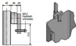
Railing post holder for the secure installation of BETOMAX® railing posts on sheet piling profiles and similar components with a material thickness of up to 27 mm.
