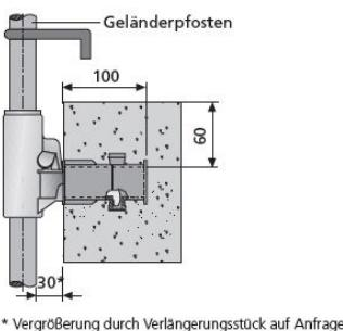
Railing post holder for holding the BETOMAX® railing post on the edges of ceilings and bridge superstructures made of concrete in conjunction with the plug socket that was concreted in beforehand.
