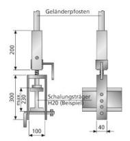
Clampable railing post holder. Suitable for wooden beams and steel profiles.
