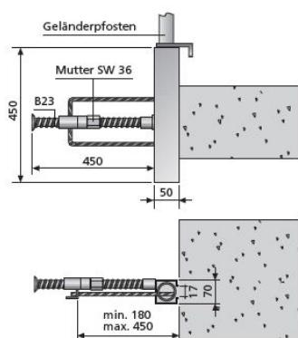
Guardrail post holder for accommodating BETOMAX® guardrail posts on the superstructure edges of bridges.
