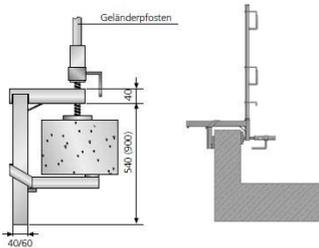
Clampable railing post holder for vertical and horizontal component edges.
