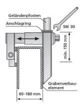
Clampable railing post holder for use on trench shoring elements. Suitable for element and wall thicknesses between 60 and 180 mm.
