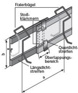
Setting up the metal water stop (SDF Q1 or Q2) on the upper reinforcement. The swelling tape must be at the bottom and fully integrated into the first concrete section
