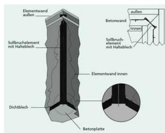
DF metal waterstops are metal sheets with a special bituminous coating for sealing horizontal and vertical construction joints.
