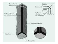
DF metal waterstops are metal sheets with a special bituminous coating for sealing horizontal and vertical construction joints.
