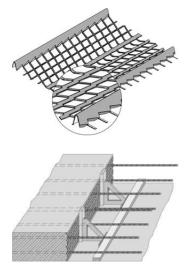
Ribbed expanded metal as permanent formwork Panel size: 2.50 m x 0.60 m =  $1.50 \text{ m}^2 (0.30 - 0.50)$
