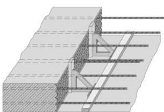
Ribbed expanded metal as permanent formwork
