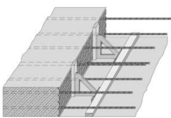
Ribbed expanded metal as permanent formwork
