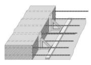
Ribbed expanded metal as permanent formwork Panel size:  $2.50 \text{ m} \times 0.60 \text{ m} = 1.50 \text{ m}^2 (0.30 - 0.50)$
