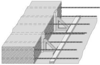
Ribbed expanded metal as permanent formwork
