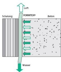
Formtex® from BETOMAX® ensures a longer lifetime for concrete structures cast in aggressive environments.
