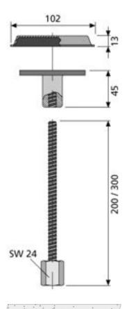
With the KNACKER®, even complicated or particularly firmly adhering bowl elements can be easily loosened. The hardened lid allows the KNACKER® to be used several times.
