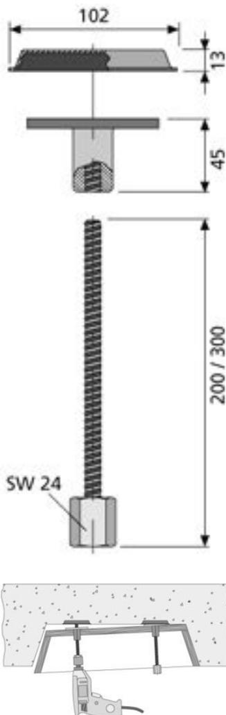
With the KNACKER®, even complicated or particularly firmly adhering bowl elements can be easily loosened. The hardened lid allows the KNACKER® to be used several times.
