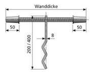
Spacer as formwork stop.
