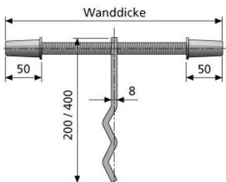
Spacer as formwork stop.
