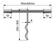
Spacer as formwork stop.
