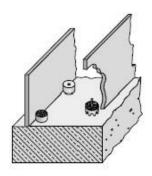
For adjusting the formwork on the underlying component.
