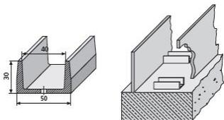
Spacer profile with nail holes for aligning and attaching wall shell elements. Instead of wooden slats, which swell and rot later. To avoid water circulation, do not arrange the base strip across the entire width, but offset.
