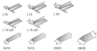
Triangular strips made of impact-resistant rigid PVC, nail flags perforated for breaking corners.
