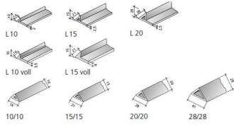
Triangular strips made of impact-resistant rigid PVC, nail flags perforated for breaking corners.
