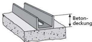
ISO-TRICK for use on soft substrates, e.g. insulated ceilings and concrete floors.
