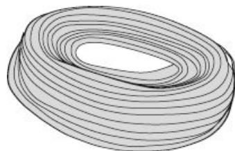
Binding wire for braiding the reinforcement.
