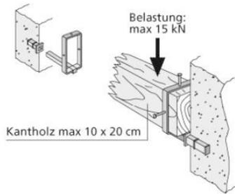
Anchorage for inserting square timbers (max. 10 x 20 cm). Use in reinforced concrete ceilings/walls/cavities, e.g. in the area of lift shafts.
