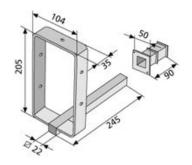
Anchorage for inserting square timbers (max. 10 x 20 cm). Use in reinforced concrete ceilings/walls/cavities, e.g. in the area of lift shafts. Permissible load: max. 15 kN
