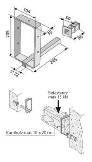
Anchorage for inserting square timbers (max. 10 x 20 cm). Use in reinforced concrete ceilings/walls/cavities, e.g. in the area of lift shafts. Permissible load: max. 15 kN
