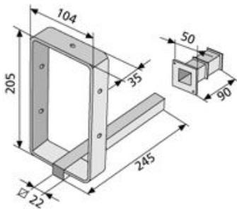
Anchorage for inserting square timbers (max. 10 x 20 cm). Use in reinforced concrete ceilings/walls/cavities, e.g. in the area of lift shafts.
