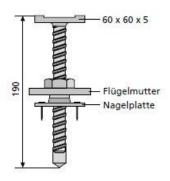
Spindle attachment for squared timber from 8 x 8 cm. Use as a clamping support, e.g. as a stop for intermediate masonry.
