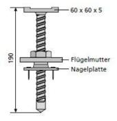
Spindle attachment for squared timber from  $8 \times 8 \text{ cm}$ . Use as a clamping support, e.g. as a stop for intermediate masonry.
