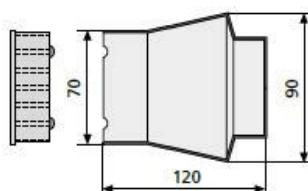
Leaves a conical hole in the concrete for inserting facade panel anchors, stone screws, etc. The thin-walled anchor box is easily pulled out of the concrete with pliers after stripping the formwork. The retaining flange is reusable.
