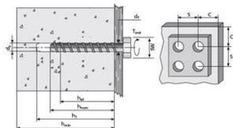
For attaching push-pull props and BETOMAX® scuffboard formwork, galvanised.
